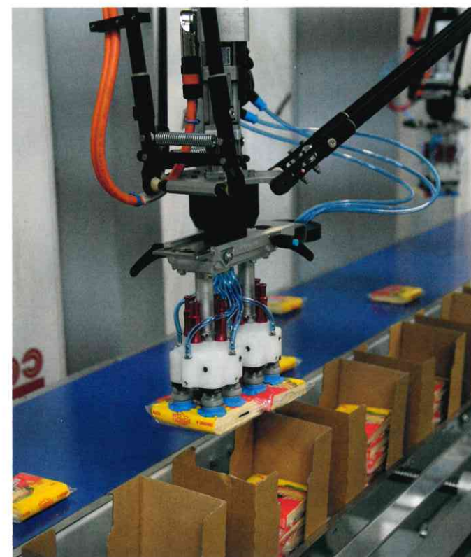
CAMA Group's packaging line with grippers using piGRIP suction cups and COAX vacuum generators (photo: Piab)
