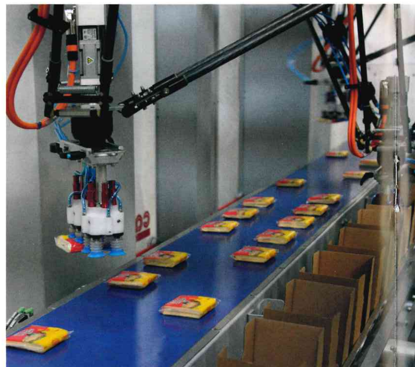
Piab's vacuum generation technology COAX minimizes energy consumption, while offering a secure and fast grip. (photo: Piab)
